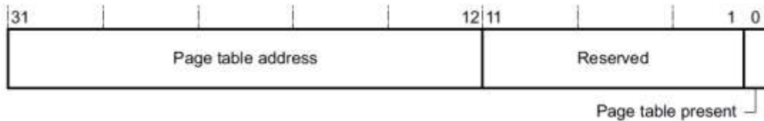
Fig. 7-3 Page directory entry bit assignments
